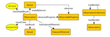
Fig. 1: A top-level, simplified schema diagram for the SOSA ontology (left) and its extension on observation collection (right).
