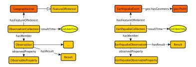
(a) Using event as the aggregator in (b) Example of using event as the ag-SOSA extension. gregator.
