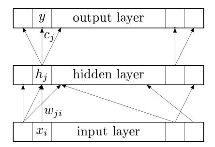
$x_i$  inputs  $w_{ji}, c_j$  connection weights y output
