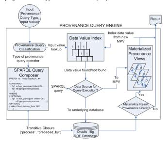
**Figure 5: Architecture of Provenance Query Engine**
